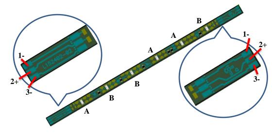
The Shine Mini Digi modules connection points has to be wired to the positive common terminal and to the function outputs of a DCC function decoder.
